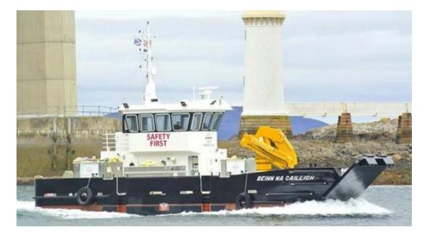
It is a workboat, constructed in the Netherlands, with two years in service as at February 2020. It is fitted with a hydraulic bow ramp and is used for ferrying personnel, materials, plant and equipment between locations. It is crewed by two MOWI employees, a master and deckhand. Mr Palmer was the master on 18 February 2020. It is nineteen metres long, with a beam of seven metres, a displacement of around ninety five tonnes and an open working deck.
